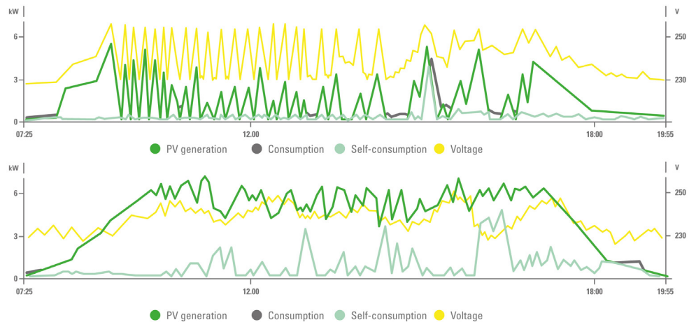
Fig. 10. Comparison of power curves and voltage fluctuations in a solar installation with U-control disabled (upper image) and enabled (lower image)
